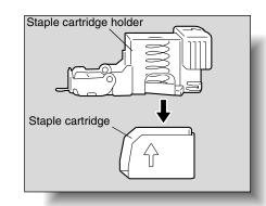
4 Insert the new staple cartridge into the staple cartridge holder.
